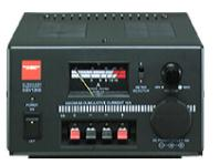
Dimensions:160Wx100Hx235Dmm Weight:5.8kg 12A(continuous)/15A(intermittent) Input voltage:AC220V 3.5A(50,60Hz) Output voltage DC1V to 15V variable Output current:12A(continuous)(13.8V) (8hours),15A(intermittent)(1 min. on and 1 min. off)
